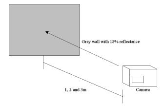
Figure 2. Experiment setup for energy table
